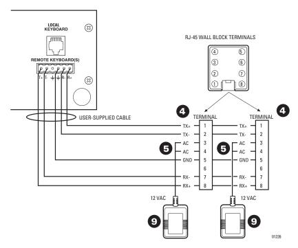
Figure 2. Keyboard Cabling Diagram
